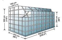
Volume: 38.0 cubic metres Standard Tare Weight: 540 kg Max Gross Weight: 13,608 kg
