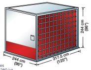
Volume: 17.5 cubic metres Standard Tare Weight: 280 kg Max Gross Weight: 6,804 kg
