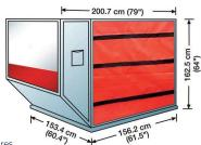
Volume: 4.5 cubic metres Standard Tare Weight: 82 kg Max Gross Weight: 1,587 kg
